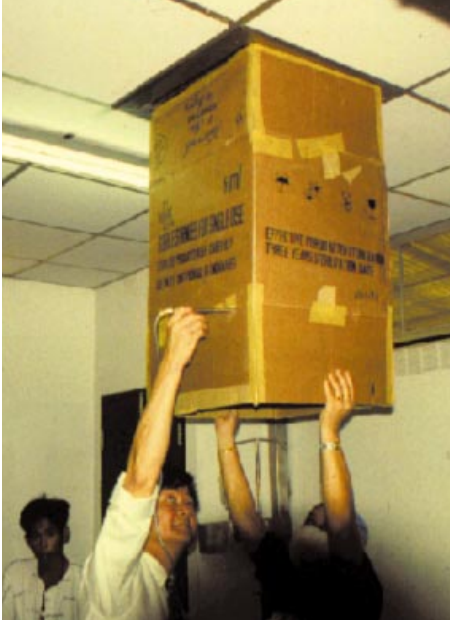
Using a carton box and flow velometer to monitor air flow in TB patient isolation room with mechanical ventilation system, Chiang Rai Hospital, Chiang Rai, Thailand
